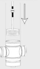
4. Cut and adjust the 250mm & 150mm PVC casings to the desired height
