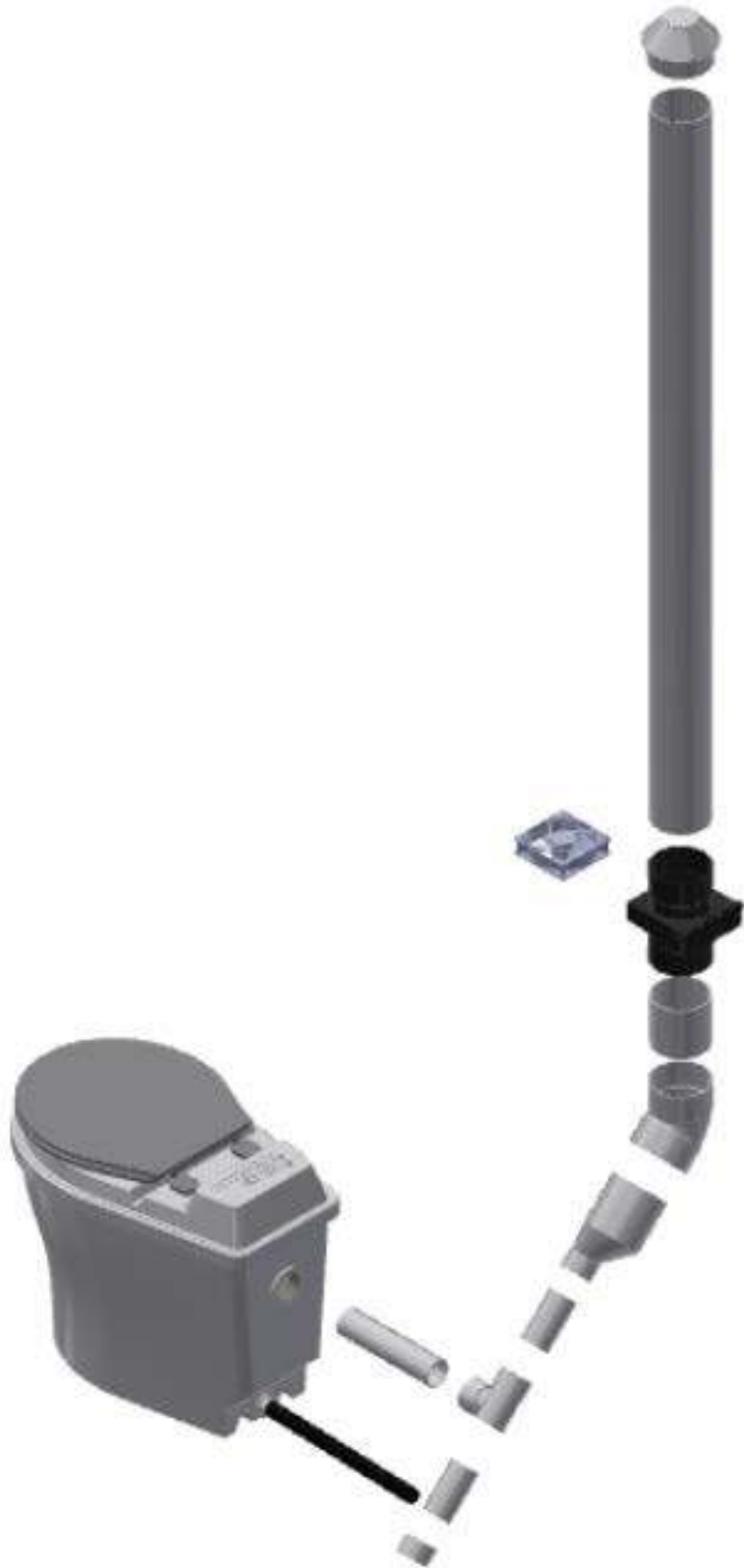
Figure 3: Ventilation pipe components break-out view
